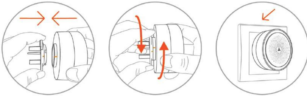
The indoor siren is powered using the mains power socket. The back-up battery is for emergency use only, when the power supply is cut unexpectedly.
